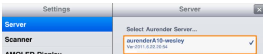
Select the Aurender Music Server by tapping its name. If no server is listed, tap Add Server at the bottom of the window and a window will appear asking for the IP address. The IP address can be found by pressing the Display Mode button on the front panel (top left) and keeping it depressed until the front display changes. Release the button. Find the IP address and enter. To return the display to the normal mode, press the Display Mode button again.
