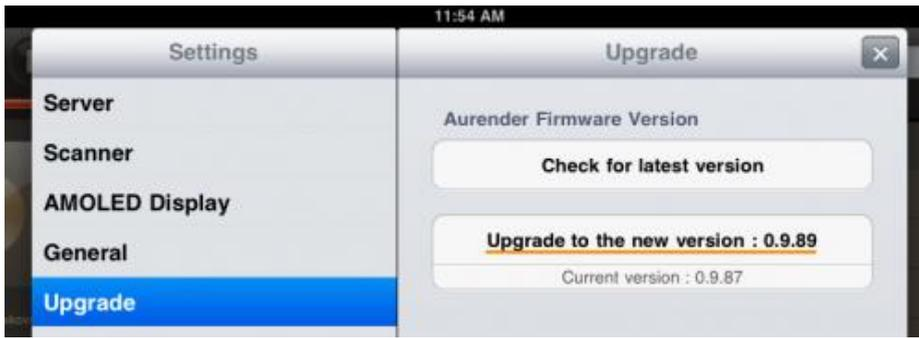
Go to Upgrade tab and check for the newest version of the music server system software and upgrade to the newest version, if needed. After upgrading, the Aurender will reboot automatically. At this time, the iPad application needs to be closed and restarted in order to be upgraded also.
