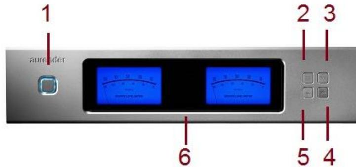
1. **On/Off** – In default mode, the power button will turn the Aurender on and off completely. The button light will stop blinking when fully turned on or off. In standby mode, the Aurender will go into standby (sleep) mode and turn on instantly. To switch to Standby mode, go to the Server tab in Settings of the iPad application. Scroll down to the bottom and turn on the “Use Standby” button.
