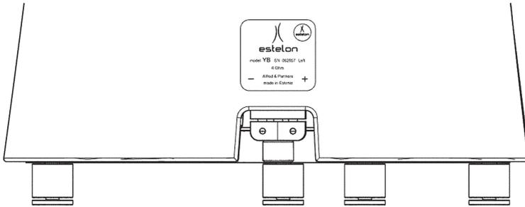
For better result we recommend connecting cables with spades. Loosen the knob, insert the both spades, then tighten the knob.
