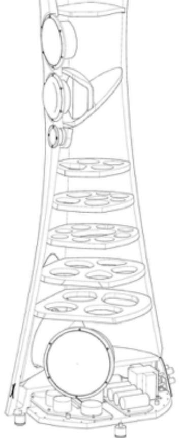
Graph 5. Internal cabinet construction showing cross-bracing and the individual chambers for the woofers, mid-woofer, midrange, and crossovers
